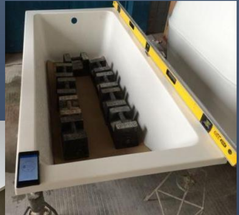
Withstand 500KGS load test, no cracking sound with this weight.
